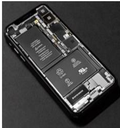
Gambar 2.9. Baterai lithium-ion (Li-Ion) (Habiburrahman, 2023)
