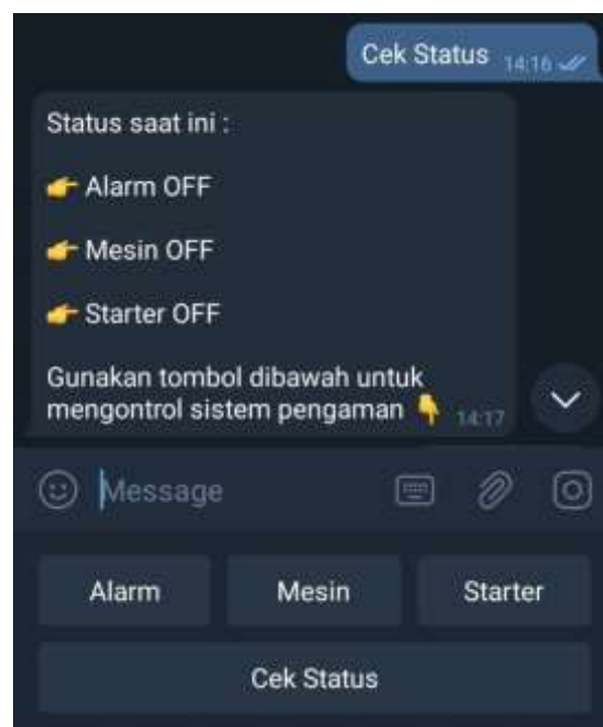
Gambar 4.23. Disain output sistem pengaman motor 1
