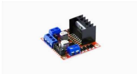
Gambar 2.8. Driver Motor L298N
