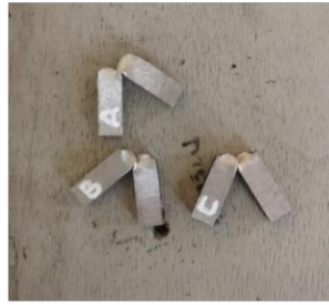
Gambar 3. 32 Hasil Uji Impact Material SS400
