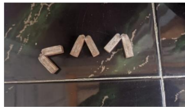
Gambar 3. 33 Hasil Uji Impact Material S 45.C
