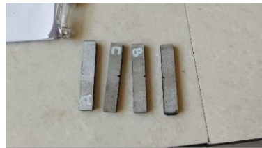
Gambar 3. 29 Hasil Spesimen Uji Impact Material SS400
