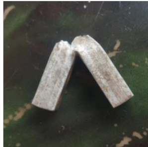
Gambar 4. 7 Hasil Uji Impact Metode Charpy Material S 45.C
