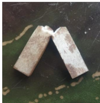
Gambar 4. 8 Hasil Uji Impact Metode Charpy Material SS 400
